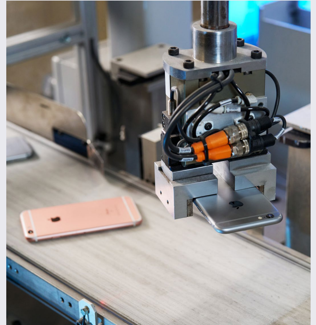
In 2023, we expanded the capabilities of Daisy, which can now disassemble 29 iPhone models into discrete components.
